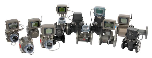
**ZENNER ZMT series** is a **MID-approved** Turbine Gas Flow Meter on-built **electronic volume converter (optional)** suited to volume measured by **turbine blade** via transmission gear by frequency transmitter (also known as pulse generator) such as Square-Wave signal (**LF**) imp. or (**HF**) high-frequency (op.) such as **Hz**.
