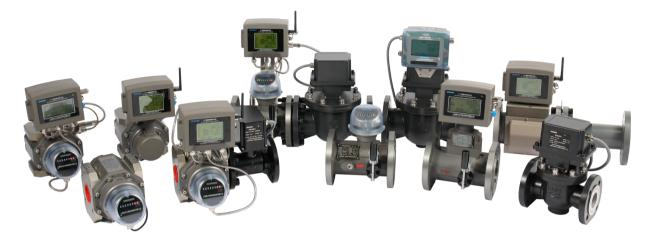
**ZENNER ZYL series** is a **MID-approved** Rotary Gas Flow Meter on-built **electronic volume converter (optional)** suited to volume measured by **displacement** via transmission gear by frequency transmitter (also known as pulse generator) such as Square-Wave signal **(LF)** imp. or **(HF)** high-frequency (op.) such as **Hz**.
